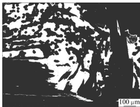
Fig.4 BSE micrograph of 3D needled C/SiC unmodified with graphite
