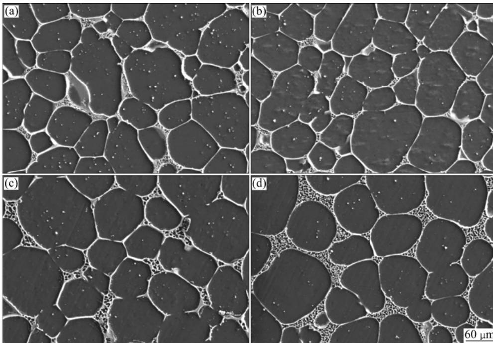
**Fig.4** SEM images of ECAE-formed ZK60+RE magnesium alloy partially remelted at 589 °C ( $\phi_s=0.8$ ) for different time: (a) 20 min; (b) 40 min; (c) 60 min; (d) 90 min
