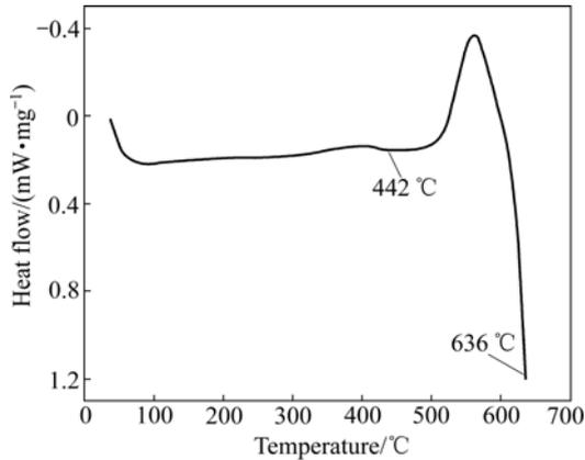
**Fig.1** DSC heating curves of as-cast ZK60+RE magnesium alloy
