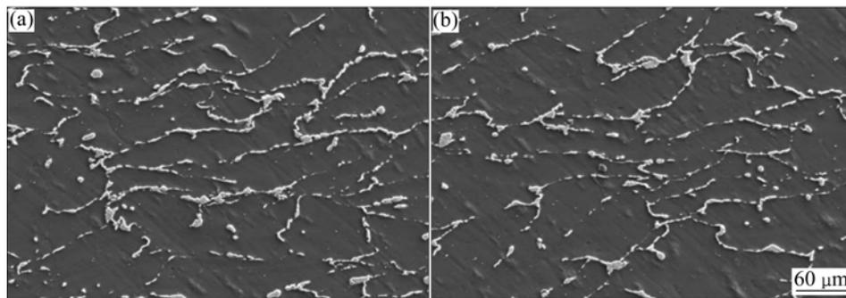
**Fig.3** SEM images of two-pass ECAE-formed ZK60+RE alloy: (a) Longitudinal section; (b) Transverse section
