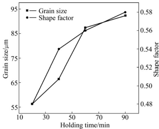
**Fig.5** Effect of holding time on mean grain size and shape factor of primary solid particles in semi-solid state
