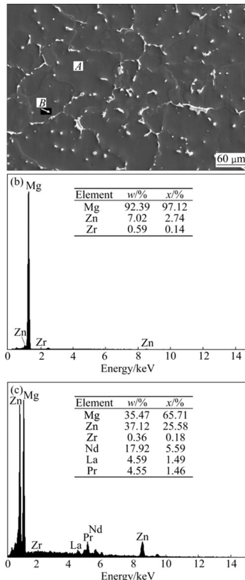
**Fig.2** SEM image (a) of as-cast ZK60+RE alloy and EDS spectra of point A (b) and point B (c) in Fig.2(a)
