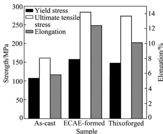
**Fig.7** Mechanical properties of thixoforged ZK60+RE components in comparison with those of as-cast and two-pass ECAE-formed ZK60+RE samples
