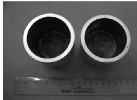
**Fig.6** Photograph of SIMA ZK60+RE alloy components
