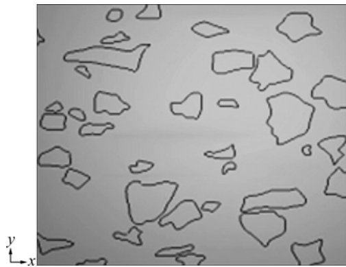
Fig.6 FEM model based on microstructure
