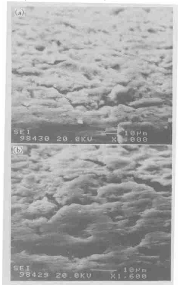
Fig.4 SEM micrographs of cross-section of eroded surfaces of composites after various treatment (a) —Treated at 500 °C for 4 h; (b) —Treated at 500 °C for 36 h
