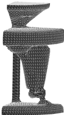
Fig.5 Gating system design and mesh generation
