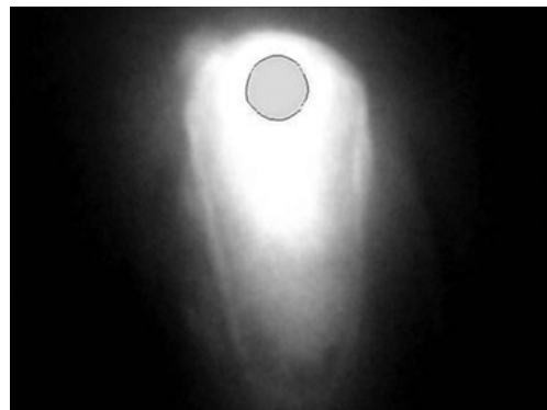
Fig.9 Keyhole edge searched by image process algorithm
